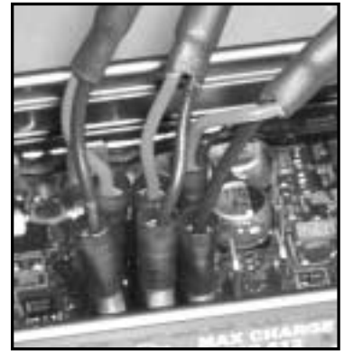
Figure 4 - Proper attachment of optional battery and alternator temp sensors at the regulator.
