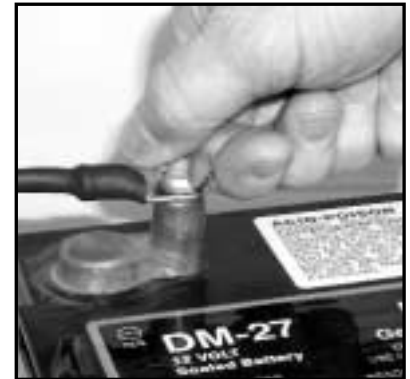
Figure 6 - Mounting temperature sensor on battery.
