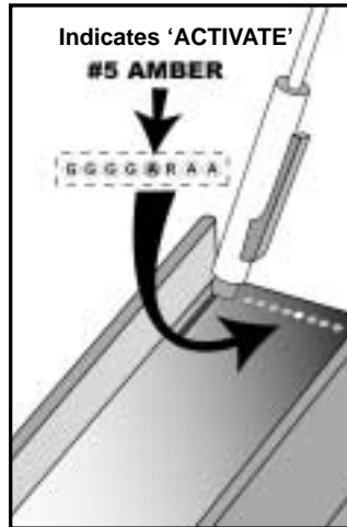
Figure 9 - Operation of magnetic reed switch.
