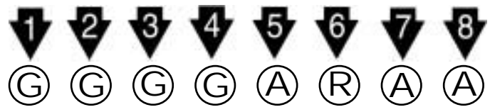
Figure 6 - Indicates system start-up.
